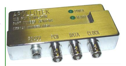
The Apollotek Model APK8764 is a general purpose PCM Simulator which is set up through a USB connection to a host PC. The unit is also powered through the USB Port. The Model 8764 is designed to work directly with the Apollotek GDSmate Telemetry Environment Software package to provide a high performance programmable PCM Simulator.
